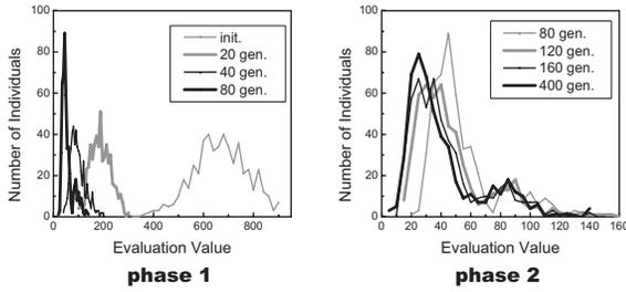
Figure 4: Search process of the GA and the distribution of the function evaluation value. Vertical axis means number of individuals in each range of evaluation value. Left figure is for phase 1 and right one is for phase 2. 'init' means 0 generation.
