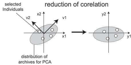
Figure 4. Reduction operation of correlation among design variables with PCA
