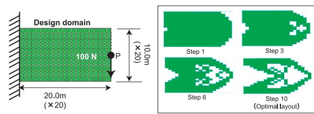
Figure 2. Evolutionary process of a structural layout using the ESO method
