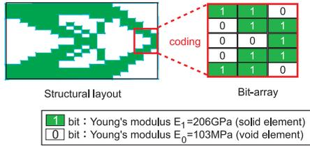
Figure 3. Coding by bit-array representation
