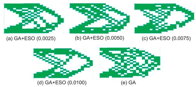
Figure 8. Final structural layout
