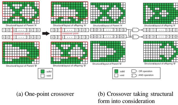
Figure 4. Comparison of structural layouts according to crossover method
