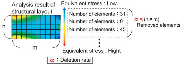
Figure 1. Removed elements of unnecessary parts using ESO method
