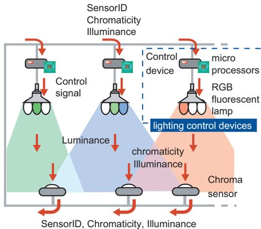
Fig. 3. Autonomous distributed lighting environment control
