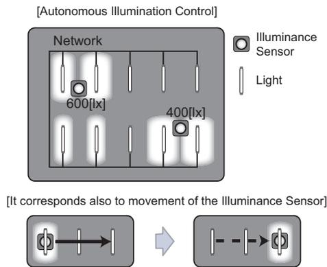
Fig. 1. Autonomous lighting control
