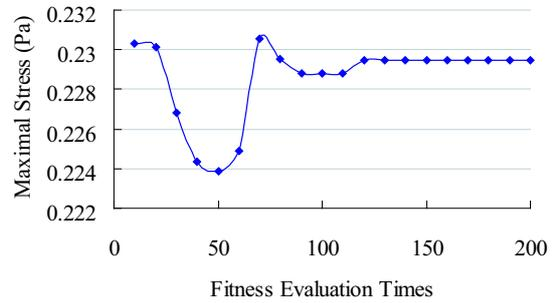
Fig.6 Maximal Stress Iteration History of Michell Problem
