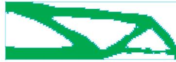
Fig.12 Final Shape of Experiment (2)
