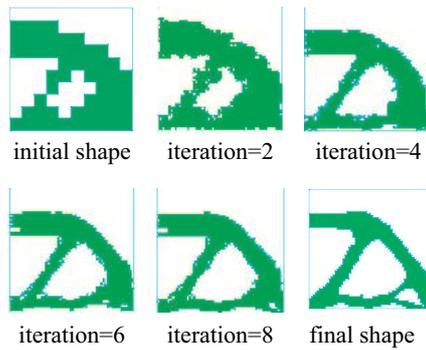
Fig. 14 Iteration History Results of Multi-Load Beam Problem
