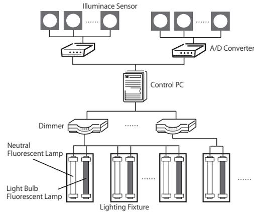
**Fig. 2.** The hardware composition for the system
