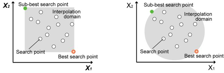
(a) Interpolation domain of hyper-cube (b) Interpolation domain of hyper-spherical
