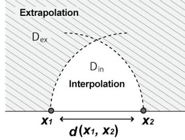
Fig. 1 Concept of interpolation and extrapolation domains
