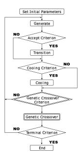
Figure 4. Flow of PSA/GAc calculation
