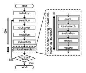
Fig. 10. The flow of the proposed GA performed in one computation node
