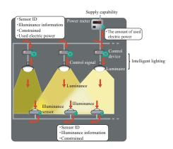
Figure 1. Configuration of the intelligent lighting system
