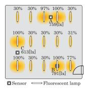
Figure 10. Luminous intensity[%] and illuminance in the stady state
