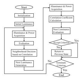
Figure 2. Adaptive Neighborhood Algorithm using Correlation Coefficient
