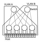
Fig. 1. VLAN-based routing method
