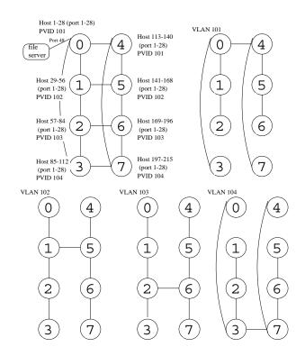
Fig. 3. Example of switch-tagged VLAN routing
