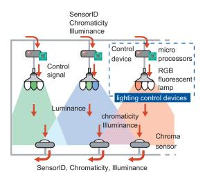
Fig. 3. Autonomous distributed lighting environment control
