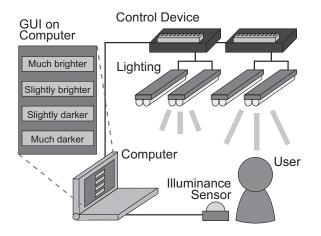
Fig. 1. Overview of the Lighting Control System through Sensory Operation
